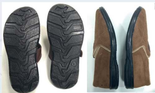
Figure. 2 Complete footwear fabricated using the injection molded PU-nanofiller composite sole
